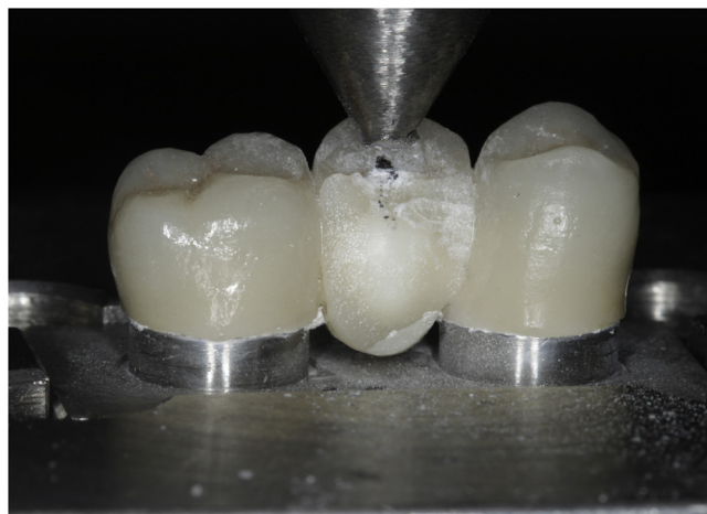
Fig. 2. ZZ restoration showing delamination of the veneering ceramic at the buccal surface of the intermediate pontic. A stepped and rough topography is discovered.
