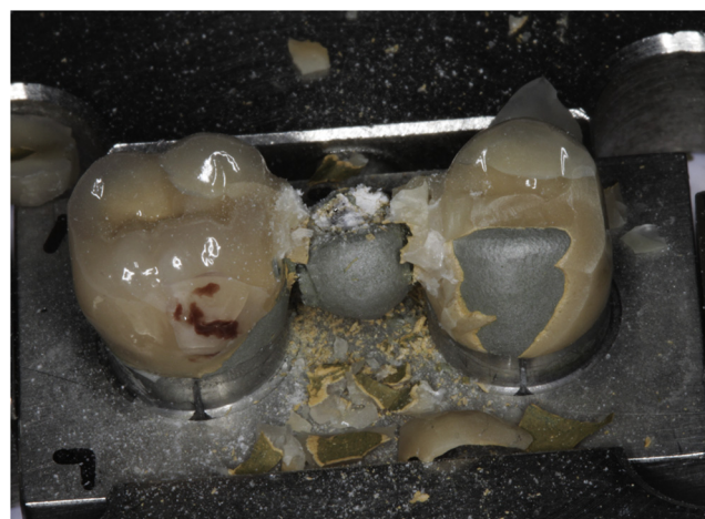
Fig. 3. Ductile fracture of a MC sample (at the connector). The plastic deformation impedes the exact fitting of the broken parts along the fracture line.
