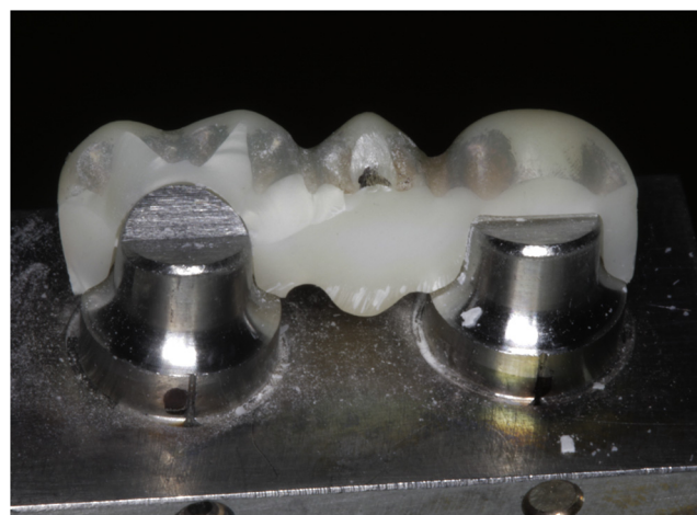
Fig. 4. LM piece fractured in half, lengthwise. The flat broken surface reveals a brittle failure.
