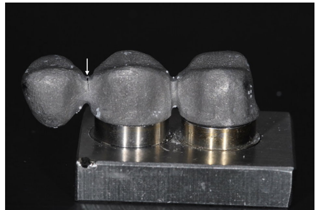
Figure 3 Fractured specimen of the soft metal milled group with cantilever.
