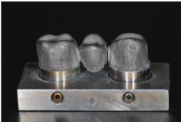
Figure 2 Fractured specimen of the soft metal milled group.
