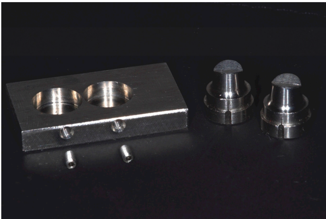
Figure 2. Master die components (platform, screws and abutments) of frameworks with cantilever pontic.
