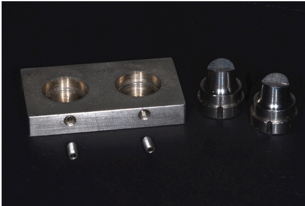
Figure 1. Master die components (platform, screws and abutments) of conventional frameworks.
